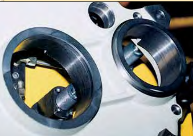
■ Lower flange work supports, placed close to the machining area to minimize deflection of the workpiece.
