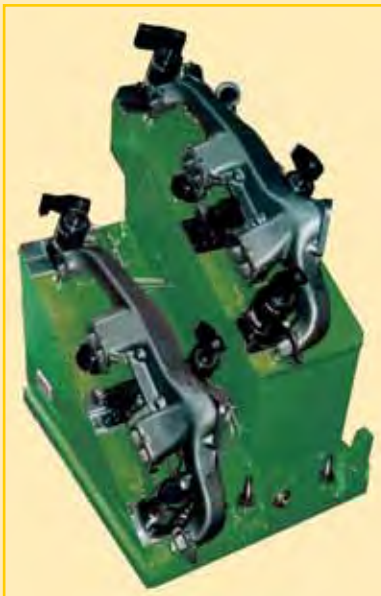
■ Fixture for machining exhaust manifolds.
