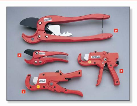
All models feature cast aluminum handles and tool steel blades for durability. These cutters are designed for cutting plastic pipe. All models feature ratcheting action to aid cutting, and feature a quick release blade mechanism to return the blade to the start position. Large cutter features long handles to provide extra leverage when cutting large diameter pipe.
