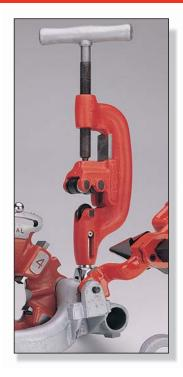
These Pipe cutters feature malleable iron frames for durability. Wide rollers help ensure blade tracking. \*Rollers can be removed and replaced with blades to speed cutting. All cutters feature replaceable cutter wheels, which can be selected to suit the application. See page 4 for cutter wheel selection chart.
